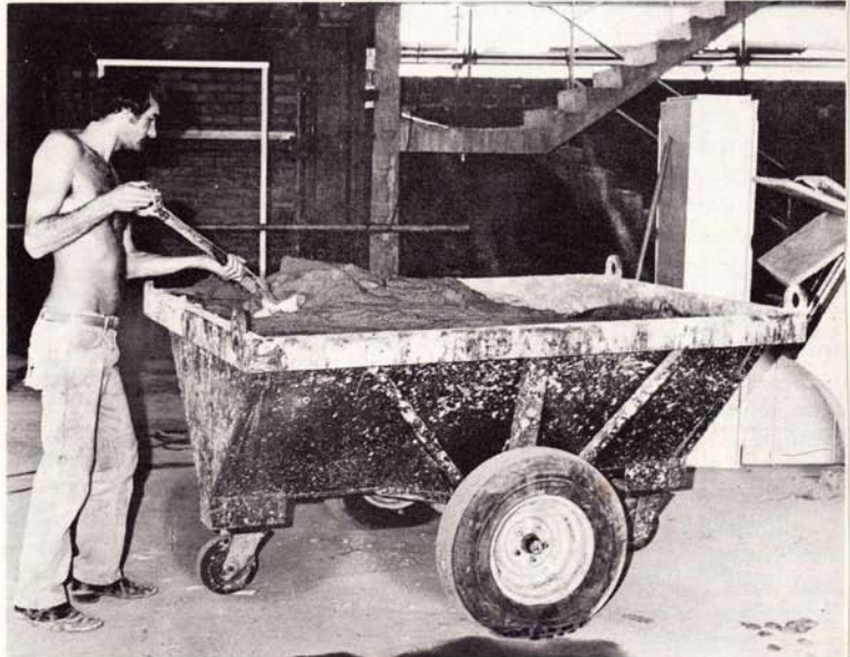
Silverwater Hire's new mobile mortar skip has corner lugs for simple attachment to crane after direct filling from concrete transport.
